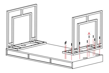
2) Align one Metal Fret End with the Drawer Box Assembly so they are flush on the end and 1/2" from the front and back edge of the Drawer Box Assembly. Using the provided Wood Screws (A), attach the Metal Fret End (10 places). Repeat Step 2 to attach the other Metal Fret End.
