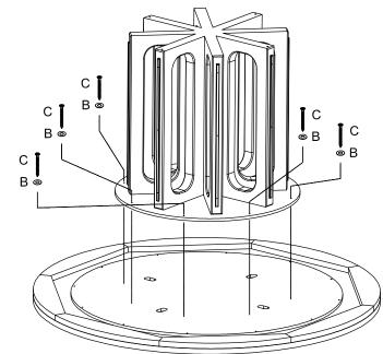
Step 3) With the top still laying on the carpet/blanket surface, use the provided screws and washers and screw through the holes into the bridge (note the grain direction of the top). Repeat for the other 3 screws.
