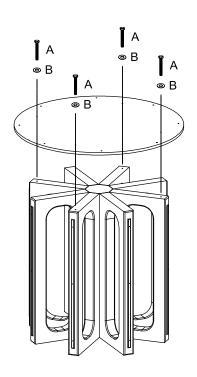
Step 2) Using provided bolts and washers, attach the bridge (that was removed in step 1) to the base.
