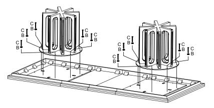
Step 3) With the top still laying on the carpet/blanket surface, use the provided screws and washers and screw through the holes into the bridge. Repeat for the other 7 screws.
