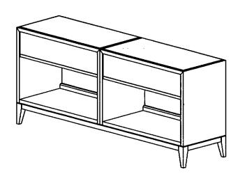
3) Using two people (one supporting each case), simultaneously lift the cases to the upright position.
