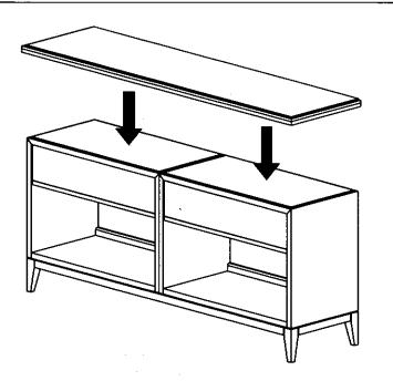
4) Lay the top panel on the top of the cases so that it overlaps both cases and flush with the back edge.
