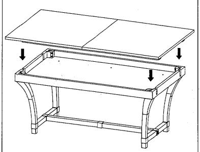
Step 5) Position Top Assembly onto the Filler Box Assembly by aligning the slides into the grooves in the end rails.
